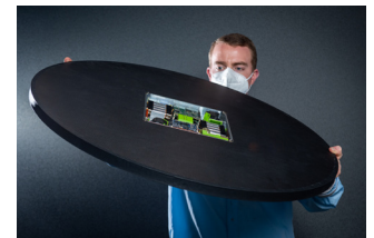
DiskSat is a plate-shaped satellite (1 meter in diameter, 2.5 centimeters thick) that could provide the required power and aperture needed for future missions.
